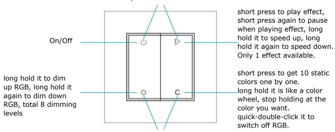
short press the 2 buttons together at the same time to turn on the 4th individual channel W, short perss them again to turn off W channel, hold the 2 buttons together at the same time to dim up W channel, hold them again to dim down W.
